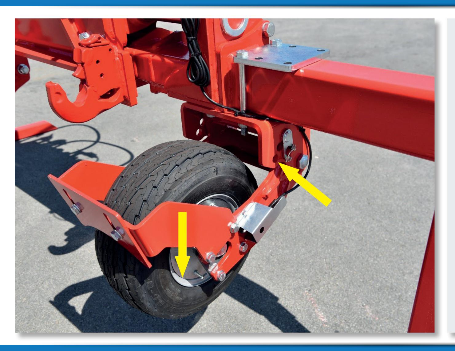
At delivery, the stabilising wheels are usually mounted at highest position.
