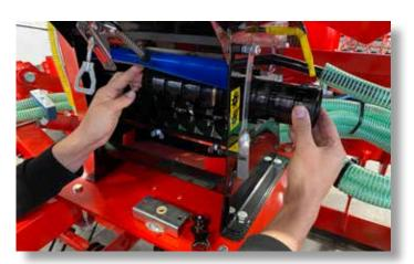
Rotation of the PTO-driven blower: up to 1000 rpm (or observe the sticker on the blower).
